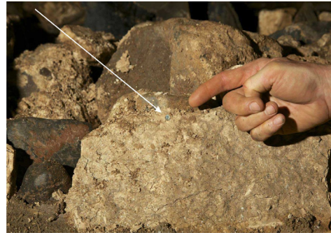
Light sensor positioned on a corner to detect light from cavers travelling in either direction
