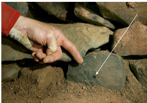
Break-beam sensor positioned where cavers are forced to walk in a trench
