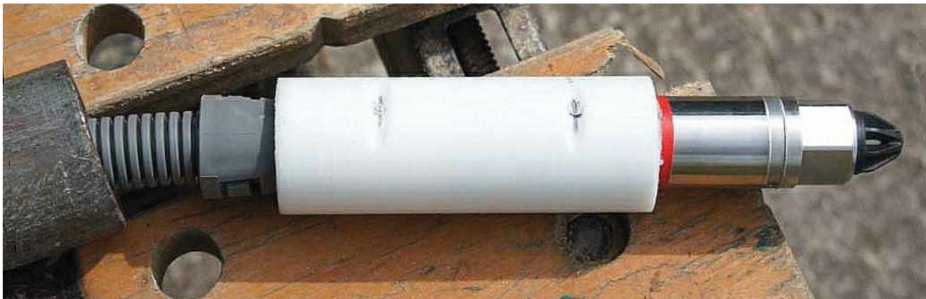
Figure 1 – Sensor in acetel tube prior to mounting in 3m scaffold pipe
