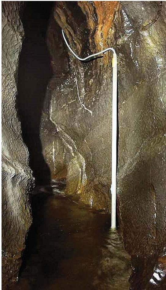
Figure 2 – 3m pipe and UNIK sensor in OFD1 streamway
