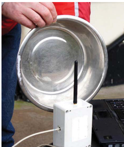
Figure 7 – Xbee transceiver at 1km range using dog bowl as reflector
