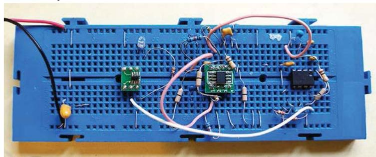
Figure 4 – The breadboarded design with ICs which are available only in SMT packages soldered to plug-in boards.
