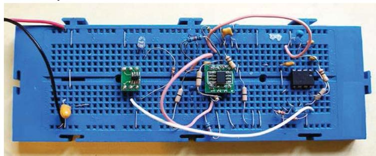
*Figure 4 – The breadboarded design with ICs which are available only in SMT packages soldered to plug-in boards.*
