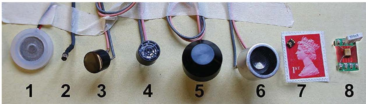
Figure 1 – Candidate bat microphone line up
